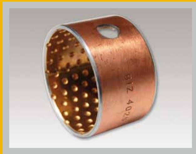
WRAPPED COMPOSITE SLIDING BEARING, STEEL/BRONZE, LUBRICATION POCKETS, LOW-MAINTENANCE
