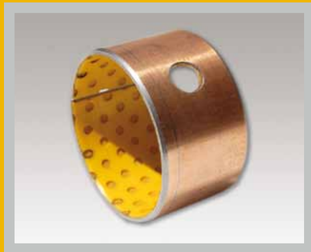
WRAPPED COMPOSITE SLIDING BEARING, STEEL/ACETAL RESIN (POM), LUBRICATION POCKETS, LOW-MAINTENANCE
